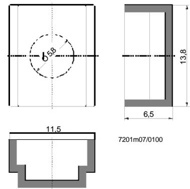
**Dummy element, small, for AGK67... cable holder**
