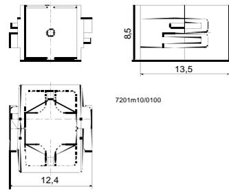
**Dummy element, large, for AGK67... cable holder**
